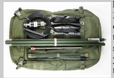
hitch mount. The base of the antenna uses a 3/8-24 thread so it can be used with a variety of mobile mounts. The system is NOT meant to be used while driving, only approved for stationary use on a vehicle. I have not tried it yet; however, I have used a mobile mount for my SuperAntenna and found the vehicle body to be ideal to use as a ground plane with no
